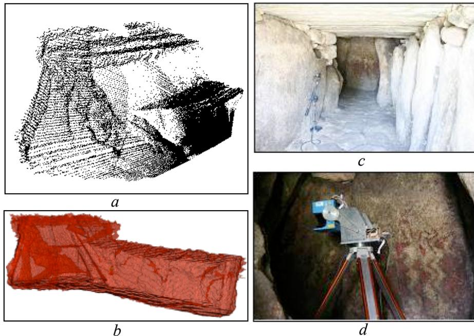
Figure 1: Acquisition of *Anta Pintada* de Antelas: (a) cloud of points; (b) Geometric model; (c,d) – Digital photographs of the acquisition..
